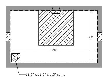
Halliday W2S7248 48" x 72" Aluminum Hatch Side View 72" 14" Ø hole 10" D.I.P 28" 4" Drain to lower elevation if possible or Sump Pump if lower elevation drain is not possible
